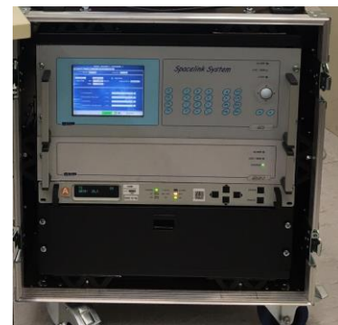
Figure 6 – NLES E5b (NAVYS, L-to-C band frequency converter, Analogic filter, RF adapter)
